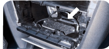
1G Skoda Octavia II Location: mounted on top of pocket behind A/C controls.
