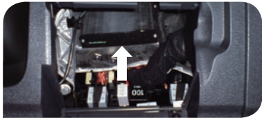
1C EOS, Scirocco, Golf V, Jetta Location: Mounted on dash support cross brace, behind driver side pocket.
