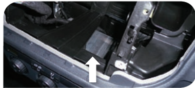
1D Tiguan Location: Attached to top of pocket, behind A/C control panel.
