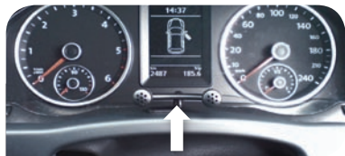
2D Tiguan Location: Attached to trim panel with wire routed behind trim panel.
