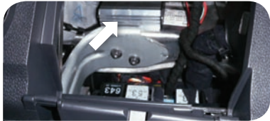
1A Golf VI Location: Mounted on dash support cross brace, behind driver side pocket.
