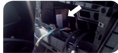
1I Skoda Yeti Location: Mounted on LHS internal wall of centre console using adhesive tape.
