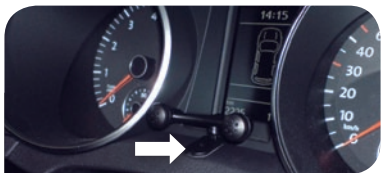
2A Golf VI Location: Attached to trim panel with wire routed behind trim panel.
