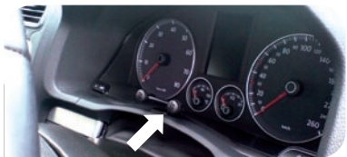
2C EOS, Scirocco, Golf V, Jetta Location: Attached to trim panel with wire routed behind trim panel.
