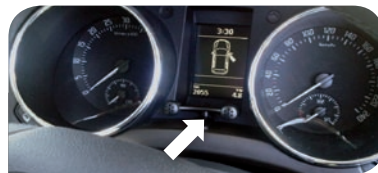
2I Skoda Yeti Location: Attached to trim panel with wire routed behind trim panel.
