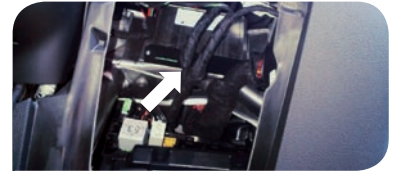
1H Skoda Superb Location: Mounted on dash support cross brace, behind driver side pocket.
