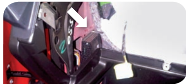
1F Polo 6R Location: Attached to LHS kick panel metal surface with double-sided tape as pictured.
