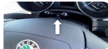
2H Skoda Superb Location: Attached to steering wheel shroud with wire routed behind vinyl cover.
