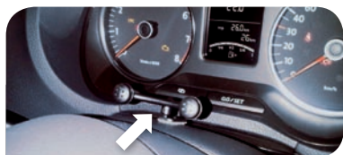
2F Polo 6R Location: Attached to steering wheel shroud with wire routed behind vinyl cover.
