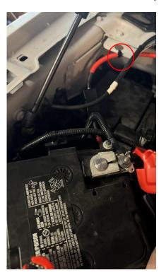
DO NOT CONNECT THE RING TERMINAL TO THE BATTERY YET!!!! WE WILL DO THIS AT THE VERY END.
