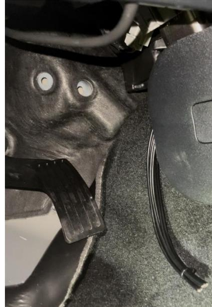
It should run alongside the power cable back to our amp in the rear.
